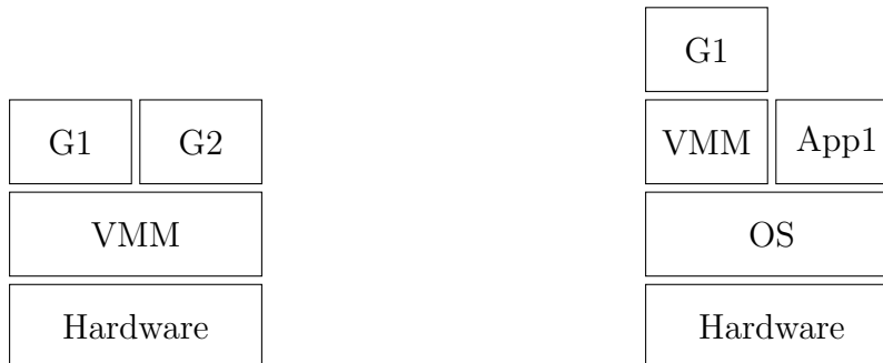
(a) Type-1 Hypervisor. A Type-1 hypervisor (VMM) executing two guest operating systems (G1 and G2). (b) Type-2 Hypervisor. A Type-2 hypervisor (VMM) executing alongside a single application (App1) and running a single guest Operating system (G1).
